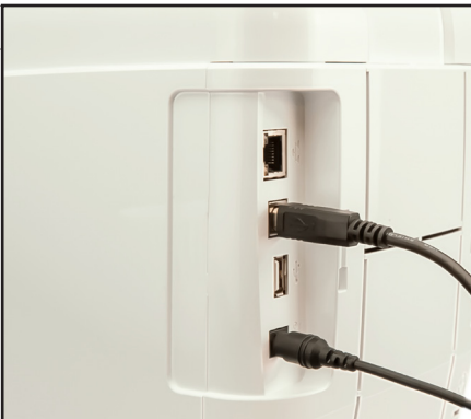
Interface for USB (high speed), built in 10/100 ethernet, Wi-Fi (optional)
